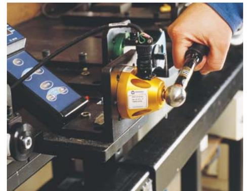
A BMX torque sensor is securely mounted for calibrating a torque wrench using a Mounting Bracket. Keeping the sensor in a stable position ensures the accuracy of the torque measurement during operation.
